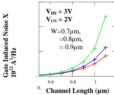
**Fig.5 Variation of Induced Gate Noise with Length for small geometry LDD MOSFETs at different device widths.**
