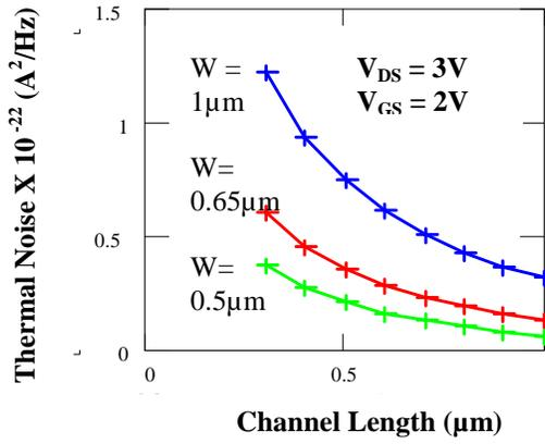
**Fig.3 Variation of Thermal Noise with Length for small geometry LDD MOSFETs at different device widths.**
