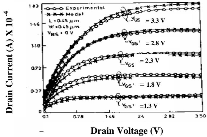
**Fig.2 Variation of drain current with drain voltage at different gate bias**
