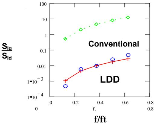
**Fig.4 Variation of  $S_{ig} / S_{id}$  with  $f/ft$  + - + - + (Model), 0 0 0 (Experimental) at  $L = 0.5 \mu\text{m}$ ,  $V_{DS} = 3\text{V}$ ,  $V_{GS} = 2\text{V}$**
